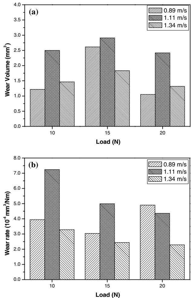
**Fig. 5 a** Wear volume and **b** wear rate of copper slid against steel in  $LN_2$  environment
