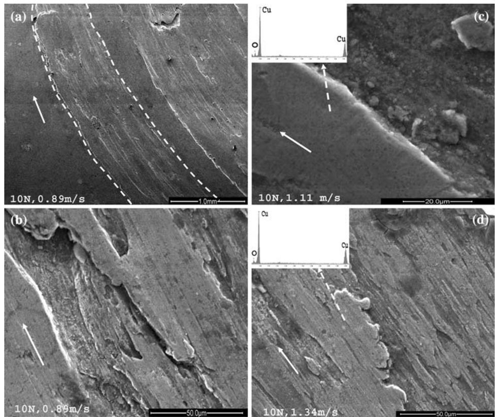
**Fig. 8** Secondary electron (SE) images of worn surfaces of copper disc after sliding at 15 N load at different speeds against steel in LN<sub>2</sub> environment. **a** Severe damage with rough surface, **b** cavity-induced delamination, **c** damaged surface and local discontinuity in tribo-layer, and **d** appearance of large cavities throughout the wear track. Arrow indicates sliding direction
