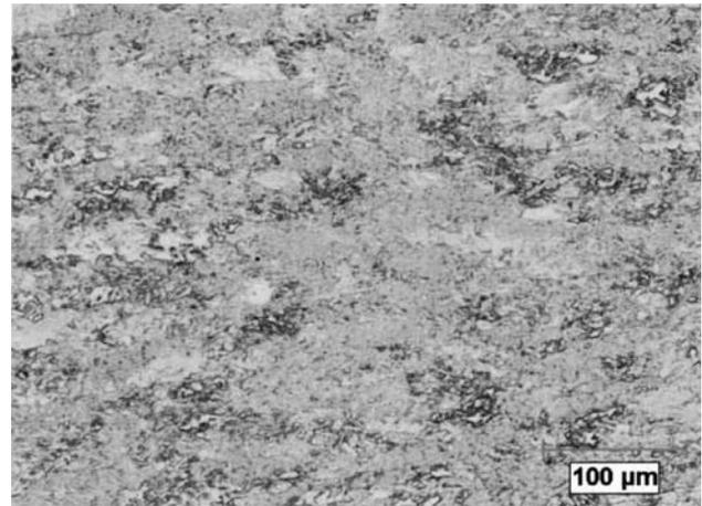
**Fig. 1** A representative optical micrograph of the copper samples used in this study. The inhomogeneity seen in the microstructure is a characteristic of the cold-worked material
