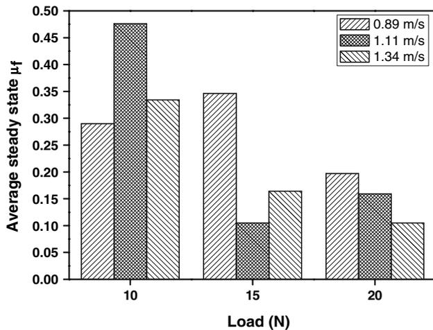
**Fig. 4** Average steady state  $\mu_F$  of copper/steel sliding couple when tested in  $LN_2$  environment
