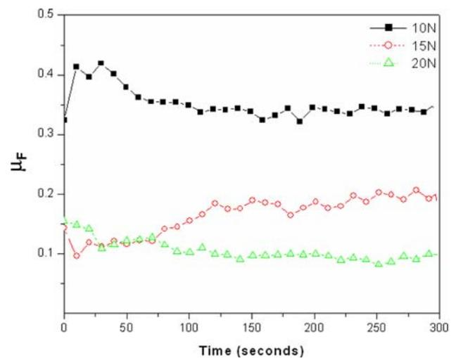
**Fig. 3** Representative plots of variation in coefficient of friction ( $\mu_F$ ) during sliding of copper against steel at 1.34 m/s speed in LN<sub>2</sub> environment
