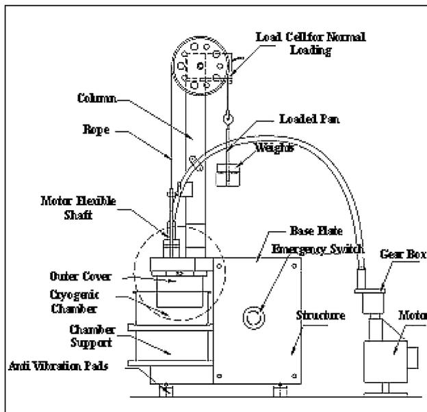
**Fig. 2** Schematic diagram showing details of the machine design of cryogenic tribometer. An important part of the machine is ball-on-flat tribological interface, which is located inside the area, marked by a dotted circle
